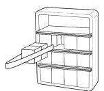
2. Finsure the tweezers blades protrude at least 35 mm outside the block. Insert the tweezers blades in the frame.
